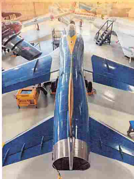
The Grumman F11F's Coke bottle shaped fuselage (K. Drewelow photo)
